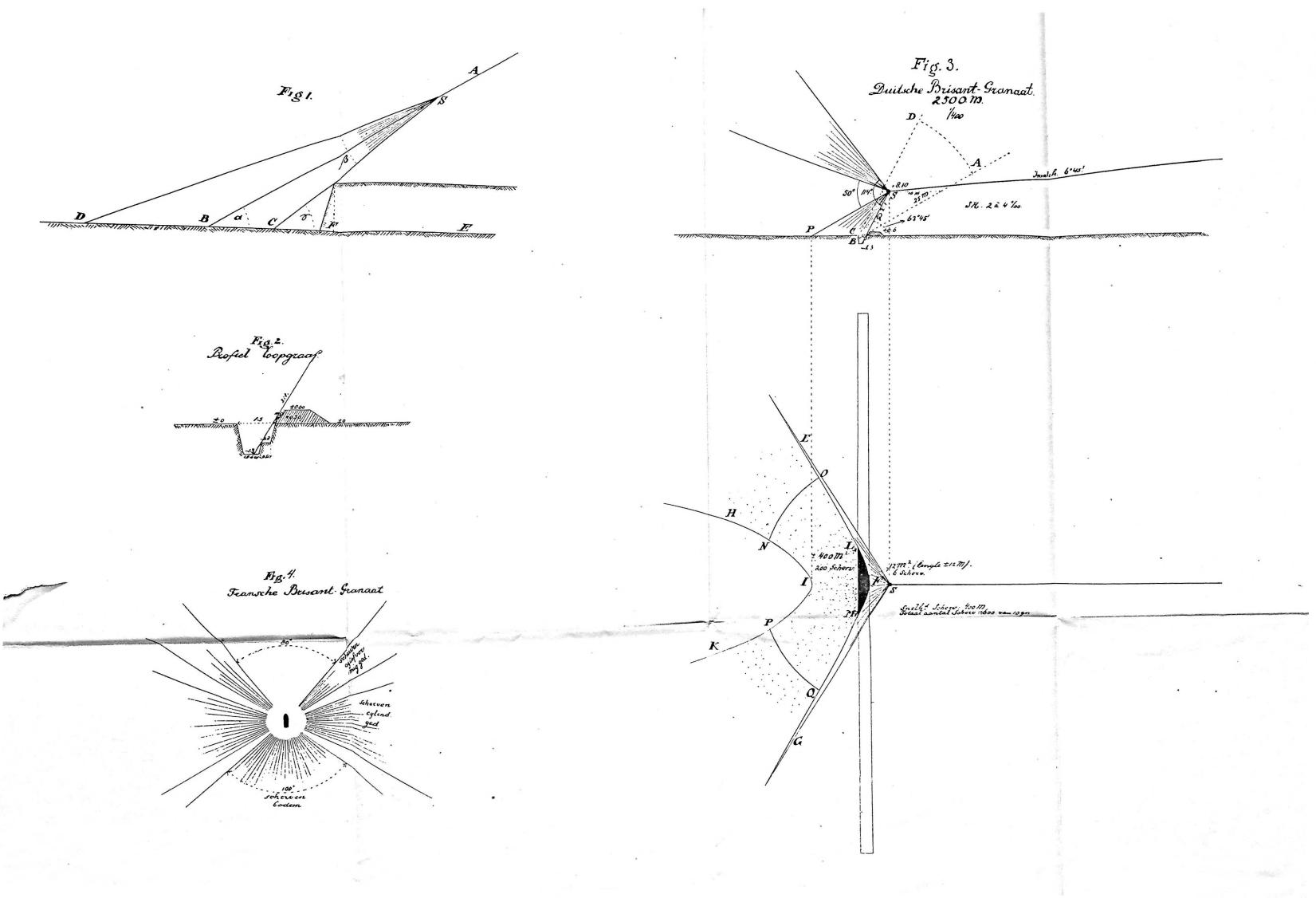
Fig. 5. Fransche Brisant Granaat. 2500 M. ±1800 m 2 ±16 \$SCHERVEN Opp ± 100M2 →LENGTE +85M
